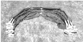
Lay the floats on the ground, place one of each length on each side of the pile of bows. With the same number of floats on each side of the bows. Making sure the black plug in the end of the float is on top. Larger covers require two or more floats to be attached to each other. If so place the ends of the floats together and with a rope tie the two together. Take the
